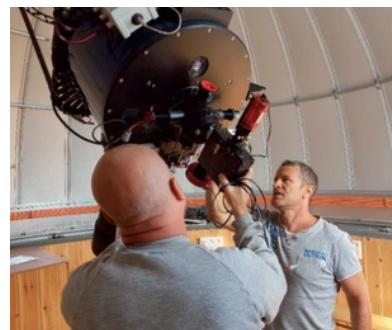
**Fig. 6.** Members of the PNST installing a spectrograph at the AstroQueyras Observatory
